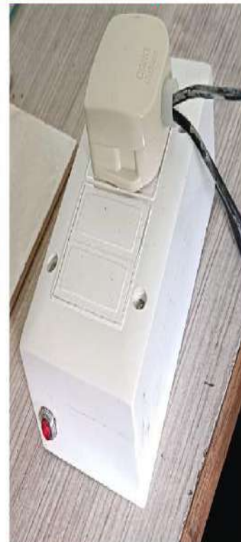
Compressor cut off device connected with sub-meter for testing
