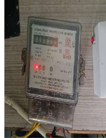
Compressor cut off device connected with sub-meter for testing
