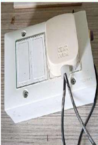
Compressor cut off device connected with Window AC
