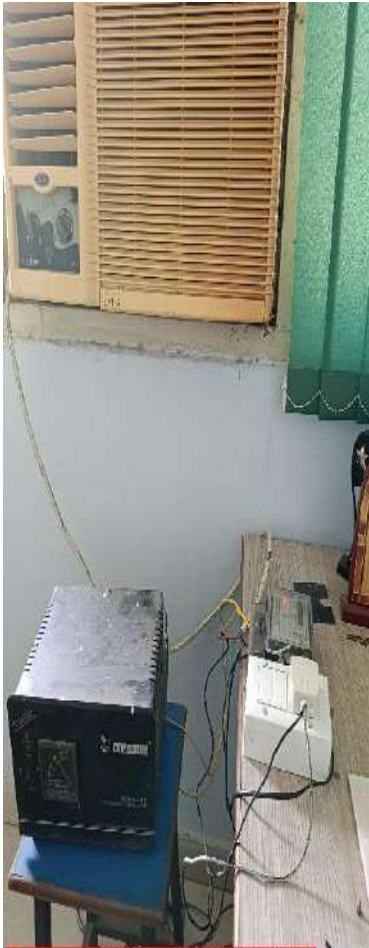
Compressor cut off device connected with Window AC
